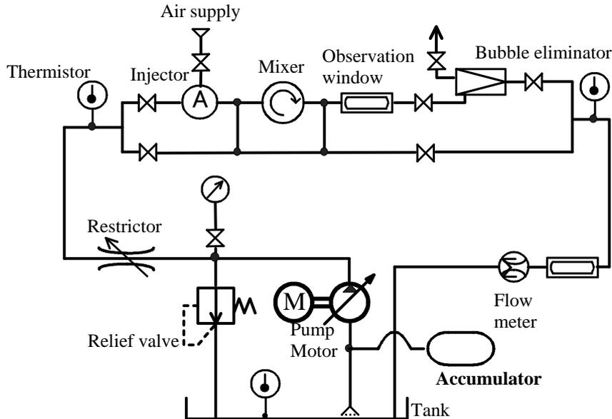
Fig.8- Test circuit for heat exchanger
