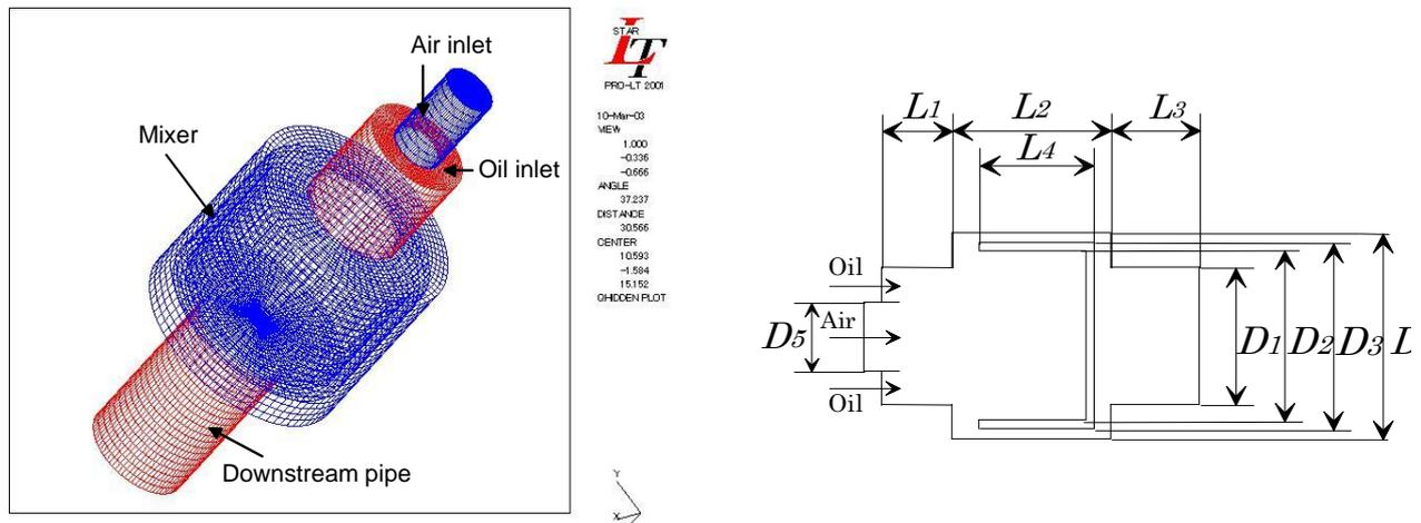
flow in the static mixer and the bubble eliminator is carried out for single-phase and multi-phase flows.
