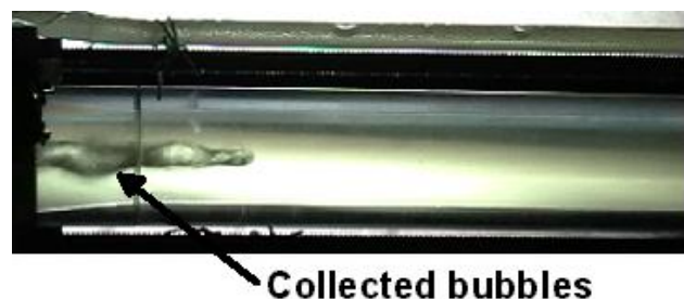
Fig.8 Flow visualization by digital video camera
