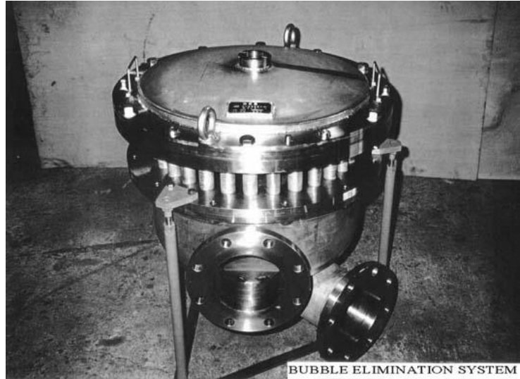
Figure1 Bubble elimination device Flow rate 2500 [L/min]
