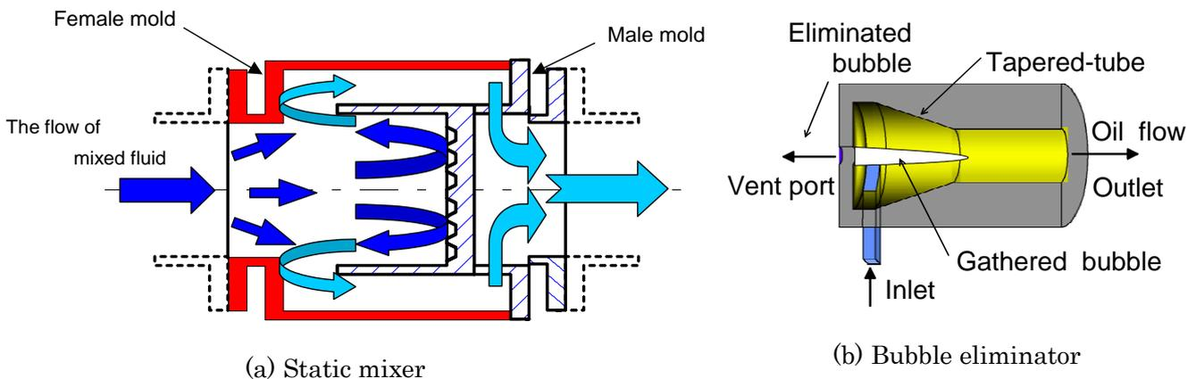
Fig.2- Principle of static mixer and bubble eliminator
