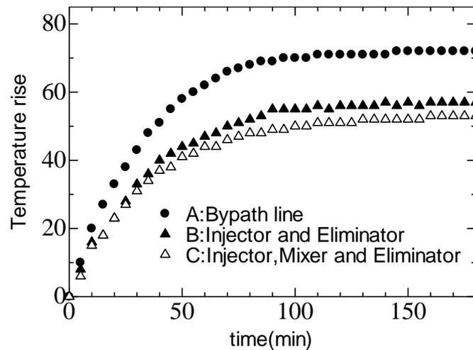
Fig.9- Temperature rise in reservoir for three test circuit conditions
