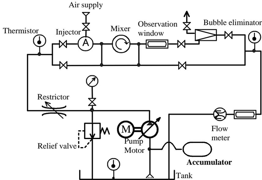
Fig.8- Test circuit for heat exchanger
