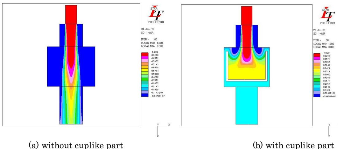
Fig.5- Simulation results of air content in static mixer
