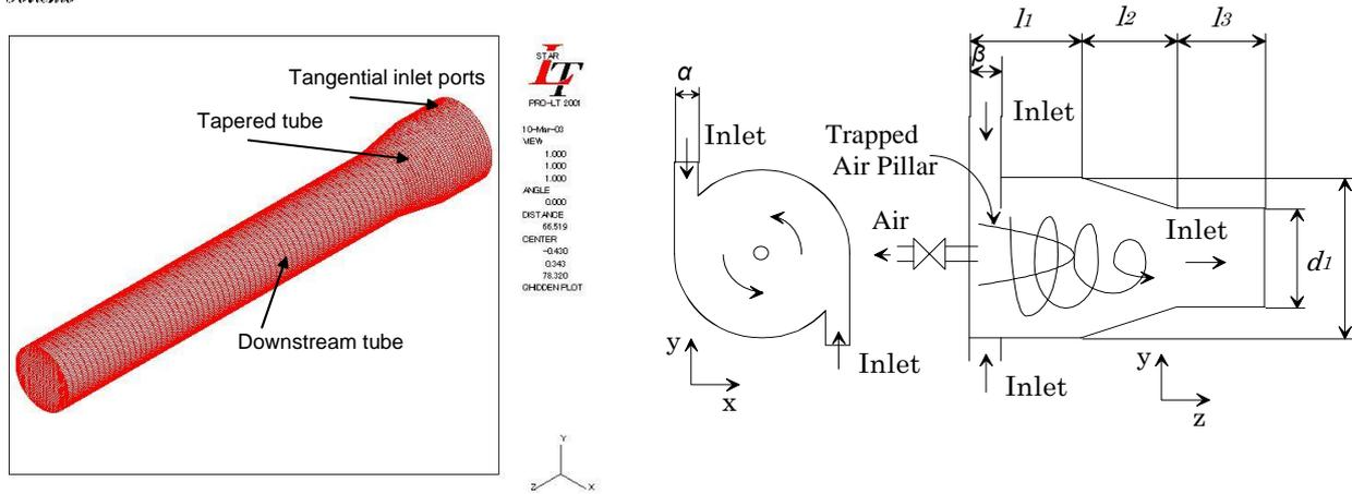
Fig.4- Mesh definition and dimensional drawing of bubble eliminator
