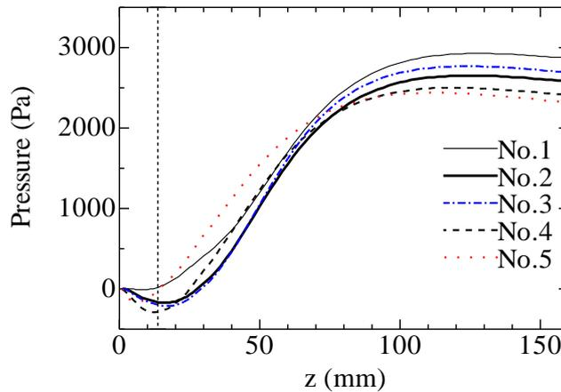
Fig.6 - Pressure distribution for the five geometric dimensions of the inlet port
